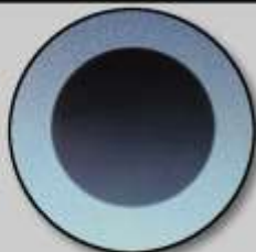
Connector after FOCCUS ™ Combination Cleaning ™
